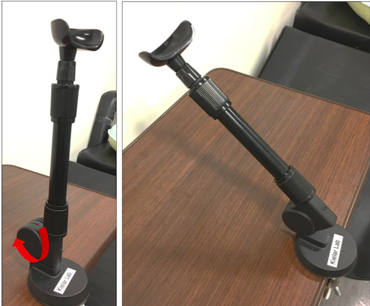
Fig. 48: Left: In its vertical position the chinrest is a good height for the average participant. It can easily be extended to be taller. If the chinrest is too tall for your participant, you can tip its angle down to any height (using the adjustment marked with the red arrow). Right: The chinrest tipped at an angle.
