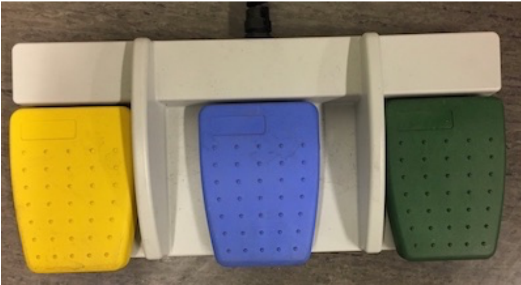
Fig. 11: 5. The Status bar along the bottom of the interface displays tiny yellow, blue and green icons that describe the footpedal functions for the active mode. These same yellow, blue and green icons appear in various control panels where they implement the same functions as the footpedals.
