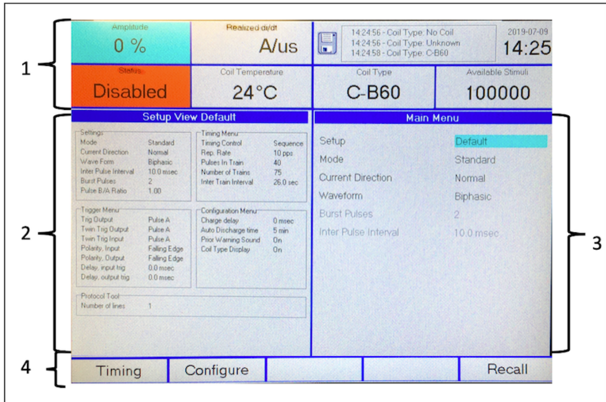
Fig. 3: MagPro Screen: 1=status area; 2=information area; 3=selection area; 4=soft key area. This figure displays the default Main screen. 1: The amplitude wheel is one way to control the amplitude of stimulation (cyan field on the upper left). The Enable/Disable button controls the Status of the coil: Disabled → Enabled . The status area consists of fixed state fields, that do not change when you switch between Main and Timing . 3: The pulse sequence name is displayed in the Setup field (cyan). The Options Wheel scrolls through the available pulse sequences. After finding the desired pulse sequence, press the Recall soft key. 4: The leftmost soft key switches to the timing menu if you wish to see details of the pulse sequence. Once in the timing menu, the leftmost soft key switches to say Main so you can switch back to the Main display when finished. You can see an example of the Timing display in the TBS section
